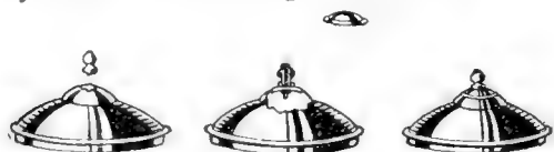
Two washers and a stove bolt used to repair the broken cover of a kettle
